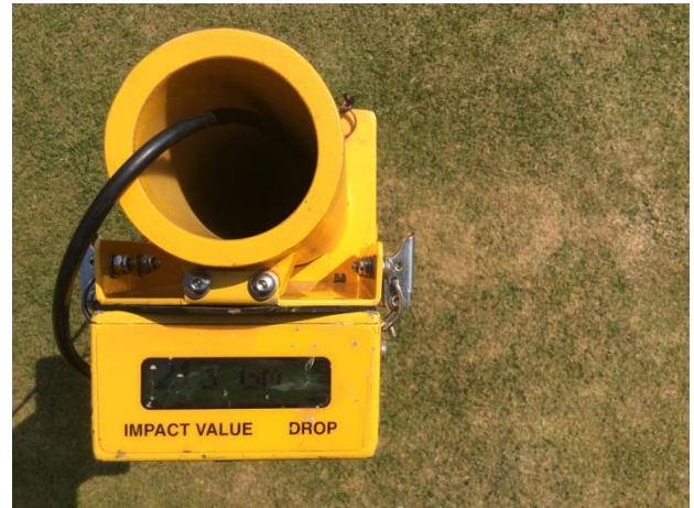
Figure 16: The result of a significant lack of moisture is that the surface effectively bakes-off which is reflected in a surface firmness reading of 213 gravities (e.g. target 120-170 gravities)
